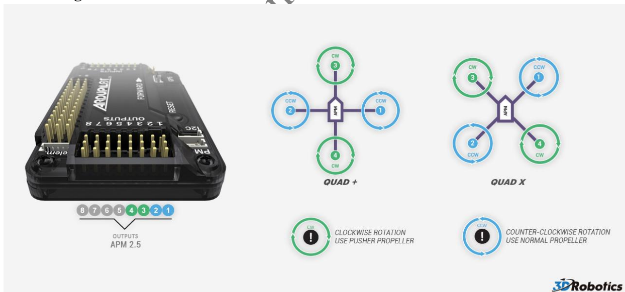
Figure 12: Connecting the Right motor and ESC to APM
