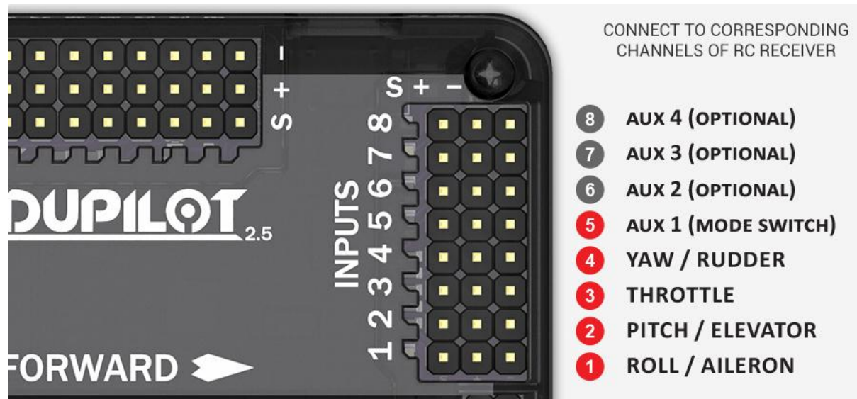
Figure 13: Connecting the Radio Receiver and APM
